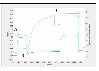
Figure 1. Immobilization of the anti-fibrinogen antibody on a MUA surface, with subsequent injections of EDC–NHS (A), Anti-fibrinogen (B) and ethanolamine (C). The antibody immobilized gives rise to a response of  $145m^{\circ}$ , which is equivalent to an amount of  $1.2ngmm^{-2}$ .
