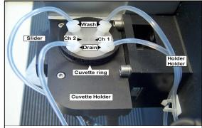
Figure 2 An overview of the cuvette holder.
