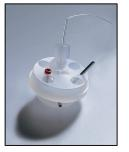
Figure 3 The electrochemical Cuvette.
