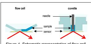
Figure 1. Schematic representation of flow cell (left) and cuvette (right) configuration
