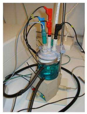
Figure 2 - Cell setup used in this application note
