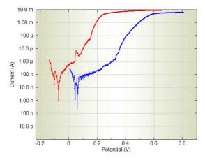
Figure 3 – Polarization curves for 304 steel recorded at  $25^{\circ}$  (blue line) and  $60^{\circ}$  (red line)
