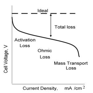
Figure 2 – i-V curve of a fuel cell showing the individual losses
