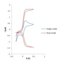
Cyclic voltammograms for 1 mM  $K_4Fe(CN)_6$  in 0.1 M KCl using single- and dual-mode at a **Platinum** IDRA electrode.
