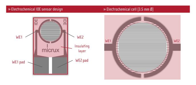
Different interdigitated electrode (IDE) designs are available in platinum or gold.
