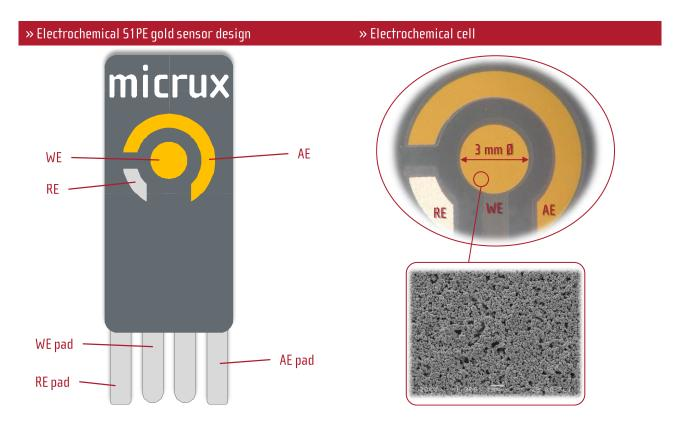
Thick-film gold-based electrodes show an excellent electrochemical behavior with a good intra- and interelectrode reproducibility. Gold-based electrodes are very useful for building *self-assembled monolayers* (SAM) and the development of *chemical sensors* and *biosensors*.
