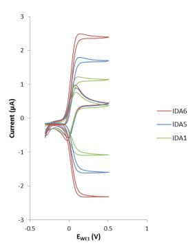
Cyclic voltammograms for 1 mM ferrocene methylalcohol in 0.1 M H<sub>2</sub>SO<sub>4</sub> using **single-** and **dual**mode at different **Gold** IDA electrodes.
