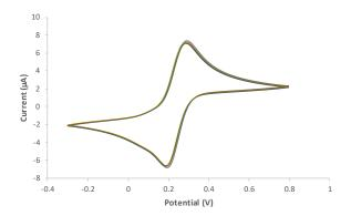
Successive cyclic voltammograms for 1 mM  $K_4$ Fe(CN)<sub>6</sub> in 0.1 M  $H_2$ SO<sub>4</sub> at the **same** thick-film carbon electrode (ED-S1PE-C10). v = 50 mV/s, n = 10, **RSD = 2%**
