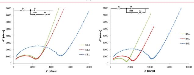
Nyquist plots using **different** gold and platinum thin-film **interdigitated electrodes** in a low conductivity NaCl solution (6.0 mS/cm). Frequencies range: 500 kHz - 100 Hz,  $V_{p-p} = 25$  mV. **Inset:** equivalent electric circuit.
