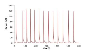
Successive injections of  $1 \cdot 10^{-5}$  M pAP in a FIA system using a thin-layer microfluidic single platinum electrode (TL-SE1-Pt). RSD = 2%, n = 13.
