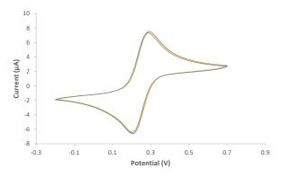
Cyclic voltammograms for 1 mM  $K_4$ Fe(CN) $_6$  in 0.1 M  $H_2$ SO $_4$  at **different** thick-film gold electrodes. v = 50 mV/s, n = 5, **RSD = 2%**
