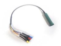
The SPE-CABLE connector *(Ref. ED-SPE-CABLE)* provides an interface between the thick-film electrodes (up to four contact pads) with the potentiostat, enabling the use of microvolume (20 –  $50~\mu L$  sample drops) or dipping into a solution. The cable ends are available with 2-mm female or male bananas.
