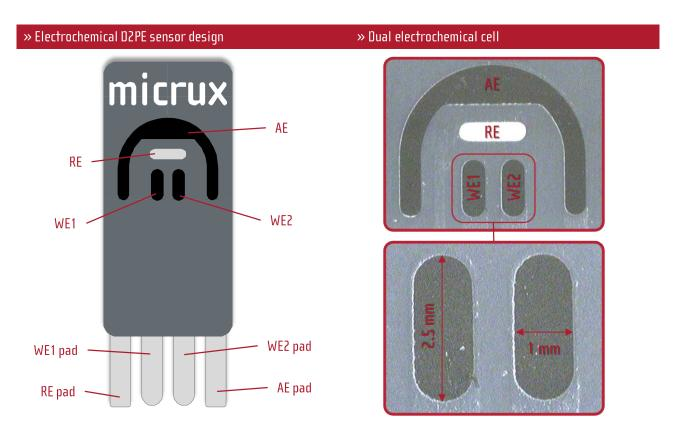
Thick-film carbon dual-electrodes show an excellent electrochemical behavior with a good intra- and inter-electrode reproducibility. Ideal for multiplexing analysis.
