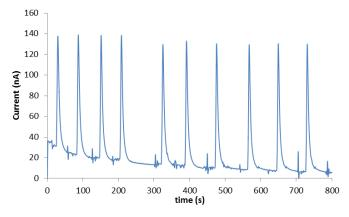
Successive injections of  $1 \cdot 10^{-5}$  M pAP in the FIA system using a thin-film Pt single-electrode (ED-SE1-Pt). Carrier: 0.1 M PBS, pH = 7.4, flow rate = 1 mL/min,  $E_d = +0.4$  V. RSD = 4%, n = 10.
