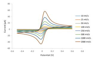
Cyclic voltammograms for 1 mM ferrocene methanol in 0.1 M H<sub>2</sub>SO<sub>4</sub> using different **scan rates** at a thick-film carbon electrode (ED-S1PE-C10).
