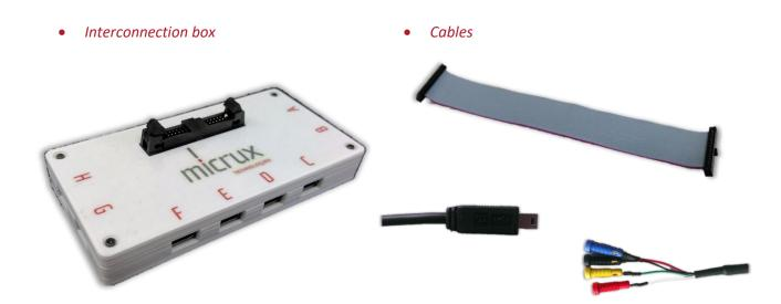
The platform enables the use of on-demand sensors, up to two 18.5x15 mm chips or one 37x15 mm chip. Tailored multi-electrode chips adapted to this platform can be manufactured with the specific requirements of the customers. The interface (connector box, cables...) for a specific multi-potentiostat can be also customized.
