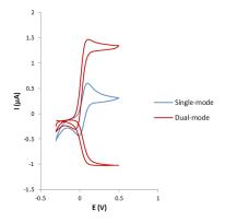
Cyclic voltammograms for 1 mM ferrocene methylalcohol in 0.1 M H<sub>2</sub>SO<sub>4</sub> using single- and dualmode at a **Gold** IDRA electrode.
