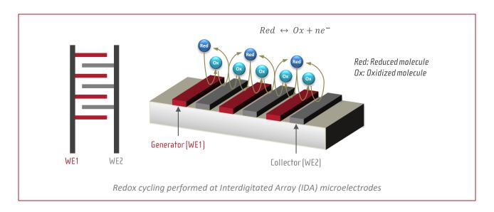
IDA microelectrode designs (width and gap) are going to affect the number of redox cycling as well as the collection efficiency.
