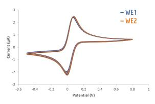
Cyclic voltammograms for 1 mM ferrocene methanol in  $0.1\ M\ H_2SO_4$  at thick-film carbon dual-electrodes.
