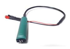
The IDE-CABLE connector (*Ref. ED-IDE-CABLE*) provides an interface between the thin-film ID $\mu$ Electrodes (IDE - two contact pads) with the potentiostat, enabling the use of microvolume (2 – 10  $\mu$ L sample drops) or dipping into a solution. The cable ends are available with 2-mm female or male bananas.
