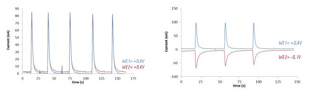
Amperometric response for  $1\cdot 10^{-5}$  M pAP in a FIA system using a **thin-layer microfluidic interdigitated array** platinum electrode (TL-IDA1-Pt) applying same and different detection potentials.
