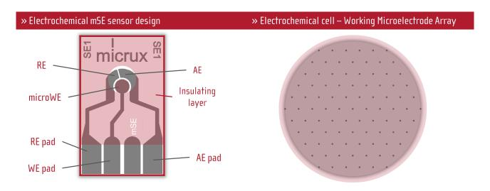
The working electrode (1 mm diameter) is based on a metal surface coated with SU-8 resin in which is defined a microholes array with honeycomb structure.
