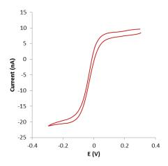
Cyclic voltammogram for 1 mM ferrocenylmethyl alcohol in 0.1 M  $H_2SO_4$  at a thin-film **gold** microelectrode array (**ED-mSE-10-Au**). v = 10 mV/s.
