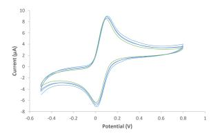
Cyclic voltammograms for 1 mM ferrocene methanol in 0.1 M  $H_2SO_4$  at the **same** thick-film graphene electrode. v = 50 mV/s
