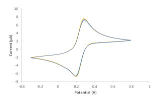
Cyclic voltammograms for 1 mM  $K_4$ Fe(CN) $_6$  in 0.1 M  $H_2$ SO $_4$  at **different** thick-film carbon electrode (ED-S1PE-C10). v = 50 mV/s, n = 10, **RSD = 2%**
