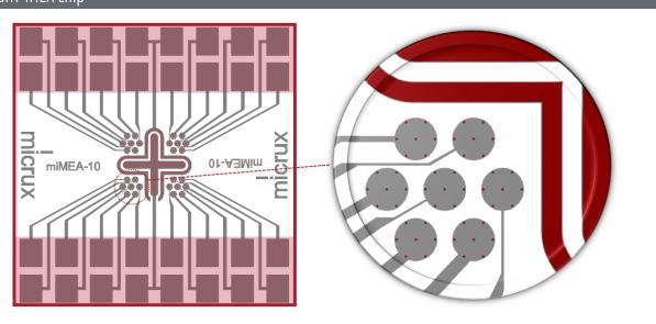
Multi-iMEA chip consists of four areas with seven sets of seven 10-µm microhole arrays (28 individually addressable microelectrode arrays) with integrated reference and auxiliary electrodes in the center of the chip.
