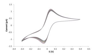
Successive cyclic voltammograms for 1 mM  $K_4Fe(CN)_6$  in 0.1 M KCl at the **same** thin-film Au electrode (**ED-SE1-AuPt**). v = 50 mV/s, n = 10, RSD = 3%
