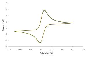
Cyclic voltammograms for 1 mM ferrocene methanol in 0.1 M  $H_2SO_4$  at **different** thick-film carbon electrode (ED-S1PE-C10). v = 50 mV/s, n = 10, **RSD = 2%**
