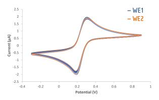
Cyclic voltammograms for 1 mM  $K_4$ Fe(CN) $_6$  in 0.1 M  $H_2SO_4$  at thick-film carbon dual-electrodes. v = 50 mV/s, n = 20 (10 + 10), RSD = 2%
