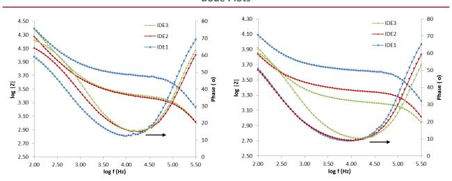
Bode plots using **different** gold and platinum thin-film **interdigitated electrodes** in a low conductivity NaCl solution (6.0 mS/cm). Frequencies range: 500 kHz - 100 Hz,  $V_{p-p} = 25 \text{ mV}$ .
