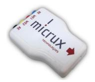
The small BOX connector (*Ref. ED-SPE-BOX*) provides an interface between the thick-film electrodes (up to four contact pads) with any kind of potentiostat, enabling the use of microvolume (20-50  $\mu$ L sample drops). The interface ends are available with 2-mm female bananas.
