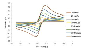
Cyclic voltammograms for 1 mM  $K_4Fe(CN)_6$  in 0.1 M  $H_2SO_4$  using different **scan rates** at a thick-film carbon electrode (ED-S1PE-C10).
