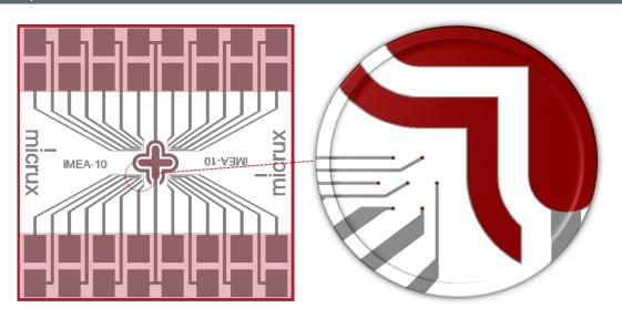
iMEA chip consists of four sets of seven 10-μm microelectrodes (28 individually addressable microelectrodes) with integrated reference and auxiliary electrodes in the center of the chip.
