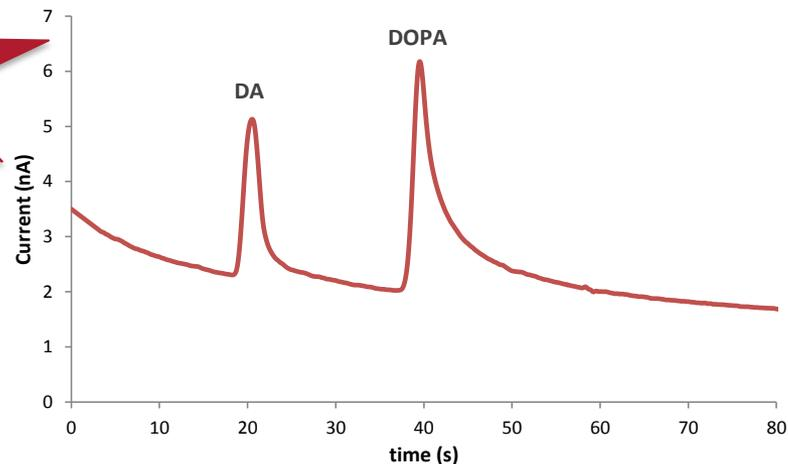
Electropherogram for the separation of 100  $\mu\text{M}$  DA and 500  $\mu\text{M}$  DOPA using a SU-8/pyrex single-channel microchip with **gold-based electrodes**. Conditions: Running buffer: 25 mM MES-His pH = 5.9;  $V_{inj} = +750$  V for 3s,  $V_{sep} = +1000$  V,  $E_d = +0.75$  V (vs. Au)
