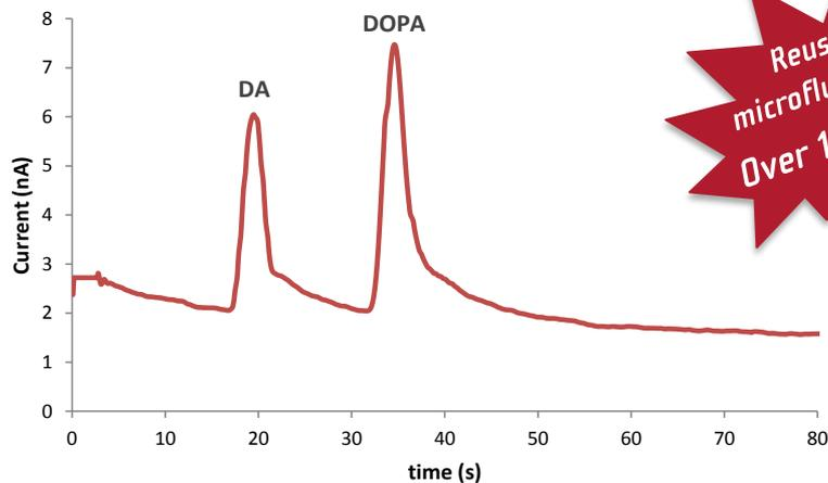
Electropherogram for the separation of 100  $\mu\text{M}$  DA and 500  $\mu\text{M}$  DOPA using a SU-8/pyrex single-channel microchip with **platinum-based electrodes**. Conditions: Running buffer: 25 mM MES-His pH = 6.0;  $V_{inj} = +750$  V for 5s,  $V_{sep} = +1000$  V,  $E_d = +0.75$  V (vs. Pt)
