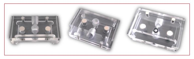
Add-on FC-PMMA-2,0 is compatible with thin-film (micro)electrodes with 2-mm diameter electrochemical cell\*. The add-on is joined to the base-cell (AIO) by means of magnets. The cell is sealed with a 2-mm I.D. O-ring. The add-on integrates standard fluidic ports (¼ " - 28 UNF) with inlet channel of 0.5 mm I.D.
