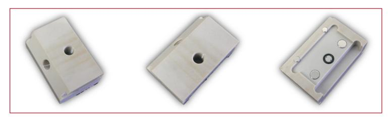
Add-on FC-PEEK-3,5 is compatible with thin-film IDµElectrodes with 3,5 mm diameter electrochemical cell\*. The add-on is joined to the base-cell (AIO) by means of magnets. The cell is sealed with a 3,5 mm I.D. O-ring. The add-on integrates standard fluidic ports (¼ " - 28 UNF) with inlet channel of 0.5 mm I.D.
