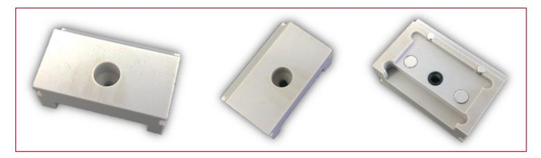
Add-on BC-PEEK-5,0 is compatible with all standard thin-film (micro)electrodes / IDμElectrodes with 2 or 3,5 mm diameter electrochemical cell\*. The add-on is joined to the base-cell (AIO) by means of magnets. The cell is sealed with a 5-mm I.D. O-ring. Sample volume up to 400 μL. \*Compatible with ED-5E1, ED-m5E1, ED-IDA1, ED-IDA5, ED-IDA6 & ED-IDRA1, ED-IDE2 & ED-IDE3
