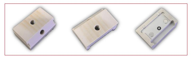
Add-on FC-PEEK-2,0 is compatible with thin-film (micro)electrodes with 2-mm diameter electrochemical cell\*. The add-on is joined to the base-cell (AIO) by means of magnets. The cell is sealed with a 2-mm I.D. O-ring. The add-on integrates standard fluidic ports (¼ " - 28 UNF) with inlet channel of 0.5 mm I.D.
