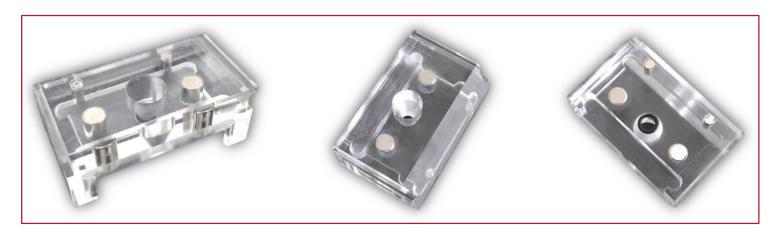
Add-on BC-PMMA-5,0 is compatible with all standard thin-film (micro)electrodes / IDμElectrodes with 2 or 3,5 mm diameter electrochemical cell\*. The add-on is joined to the base-cell (AIO) by means of magnets. The cell is sealed with a 5-mm I.D. O-ring. Sample volume up to 400 μL. \*Compatible with with ED-5E1, ED-MSE1, ED-IDA1, ED-IDA5, ED-IDA6 & ED-IDRA1, ED-IDE2 & ED-IDE3
