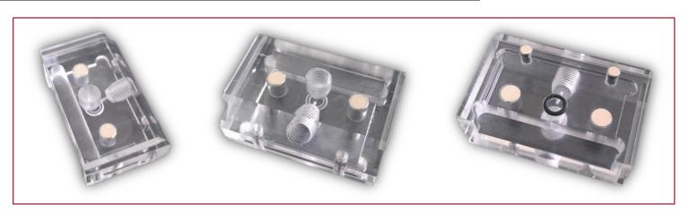
Add-on FC-PMMA-3,5 is compatible with thin-film IDµElectrodes with 3,5 mm diameter electrochemical cell\*. The add-on is joined to the base-cell (AIO) by means of magnets. The cell is sealed with a 3,5 mm I.D. O-ring. The add-on integrates standard fluidic ports (¼ " - 28 UNF) with inlet channel of 0.5 mm I.D.
