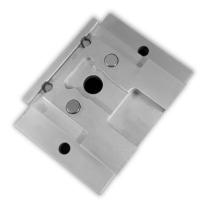
The AIO-SPE cell consists of a supporting base containing the accommodation for placing the standard thick-film electrodes (27.5 x 10.1 mm). The supporting base also includes the basic assembly parts for the different add-ons.
