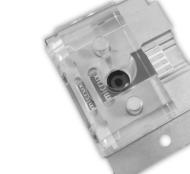
The batch-cell add-on enables the use of the standard (27.5  $\times$  10.1 mm) thick-film electrodes in applications (batch analysis, standard additions, etc...) in which are required larger sample volume up to 1 mL.
