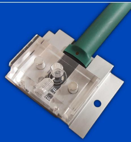
All-in-One SPE platform for thick-film electrodes
