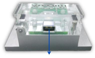
Integrated easy-to-use connector (miniUSB-type connector) with pogo-pins
