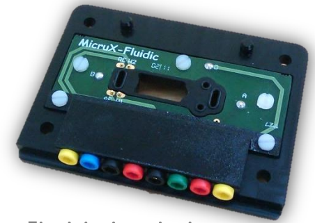
Electrical contacts on integrated PCB & 2-mm female bananas
