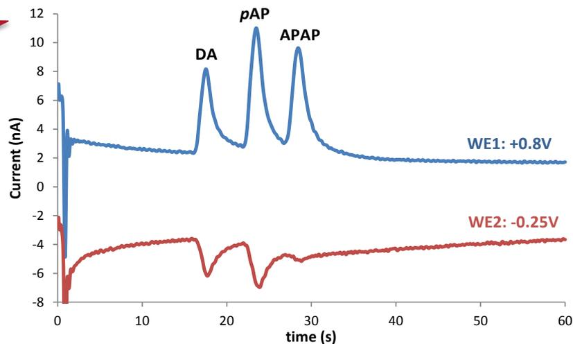
*Electrochromatograms for the separation of 100 μM DA, 100 μM pAP and 250 μM APAP using a SU-8/pyrex single-channel microchip with an interdigitated array microelectrode applying same and different detection potentials.*
