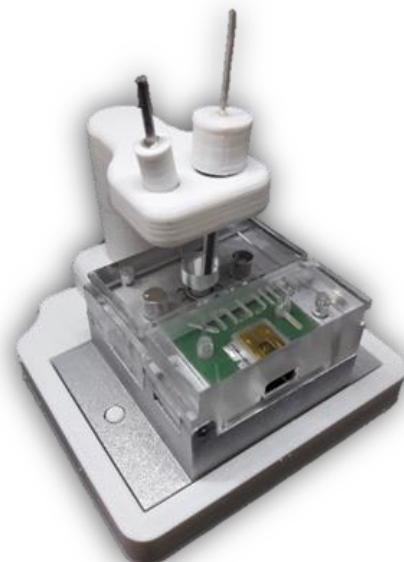
Platform with external reference & auxiliary electrodes
